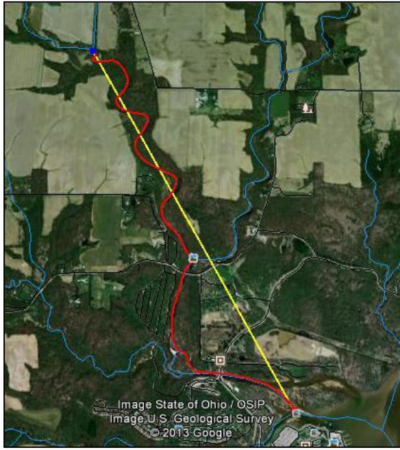
Figure 22. Google Earth image of the Four Mile Creek (red) and the total distance between two points (yellow), used to determine the sinuosity of the stream.
